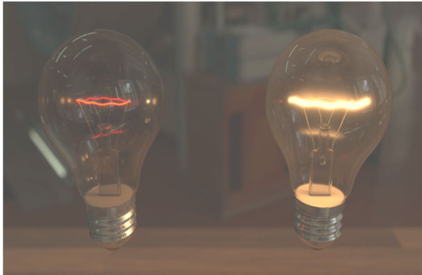
Thermal radiation in light bulbs at different temperatures
